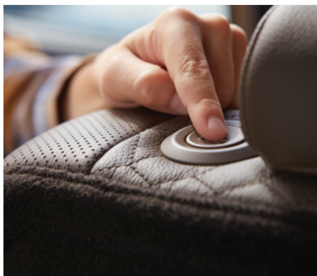
One-Touch Folding The one-touch folding feature allows you to fold the 2nd row seat easily by the push of a button.
