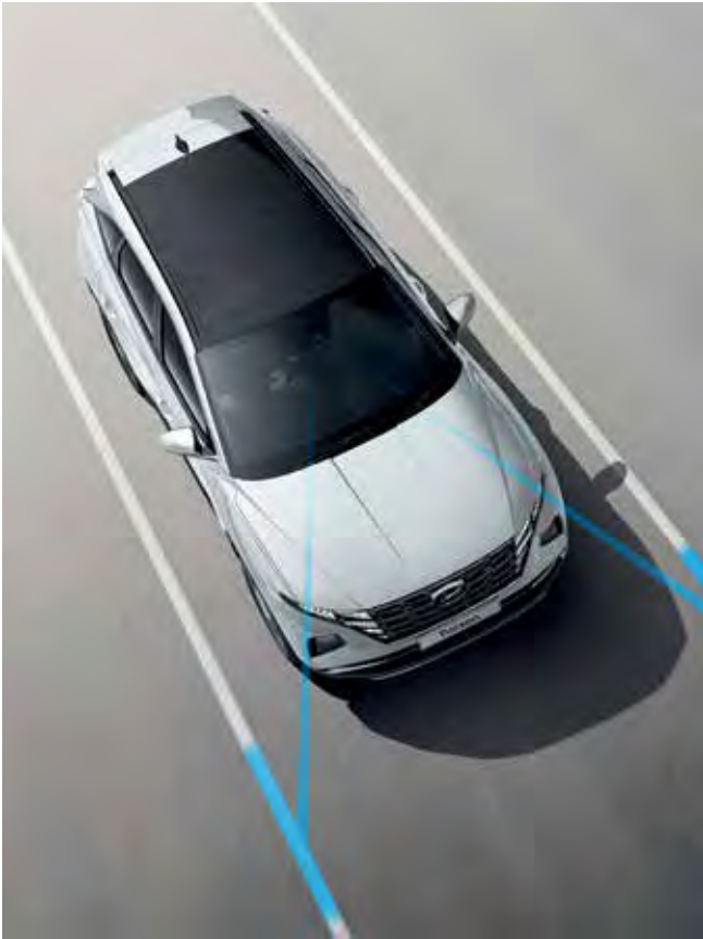
Lane Following Assist (LFA) LFA keeps you centered within the lane using its front view camera to monitor lane markers.
