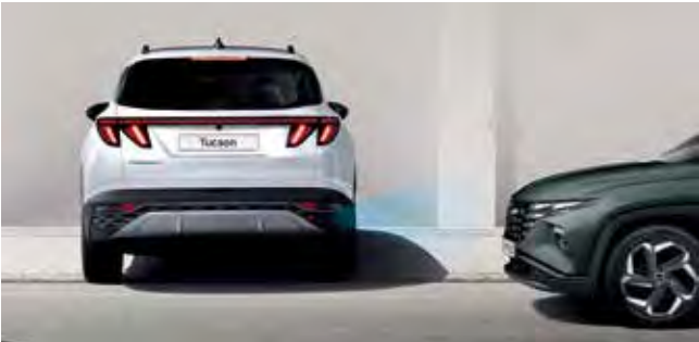
Rear Cross-traffic Collision Avoidance (RCCA) When backing out, RCCA warns the driver to the approach of a vehicle crossing their rearward path; if necessary, the emergency braking is automatically applied to avoid a collision.
