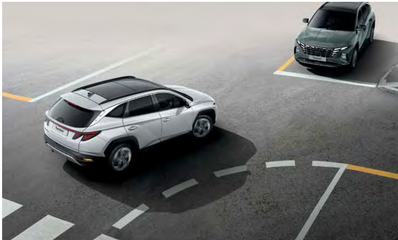
Forward Collision-Avoidance Assist (FCA, Junction Turning) FCA capabilities have been expanded to include Junction Turning function. While driving if there is a risk of collision with an oncoming vehicle while turning right at an intersection, the function automatically assists with emergency braking.
