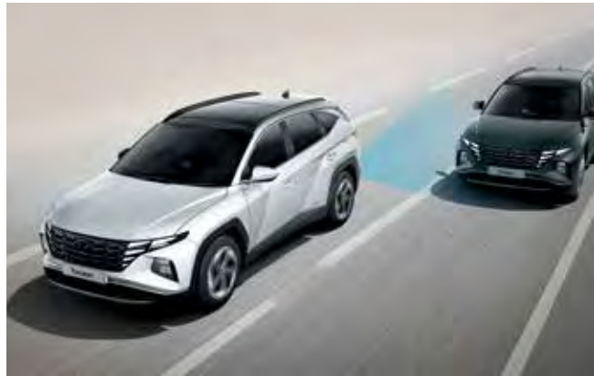
Blind-spot Collision-Avoidance Assist (BCA) BCA uses rear corner radar to monitor both of your blind spots. If a vehicle is detected in the blind spot while the turn signal is flashing, BCA will automatically apply differential braking during your attempted lane change thus helping you avoid an unsafe lane change and a potential collision.
